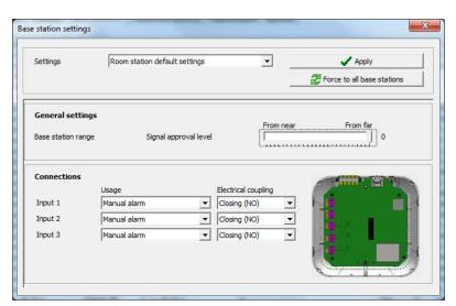
open) or "opening" (normally closed). For example, a door connection is usually NC because the door is normally closed and an alarm should be generated if it is opened.
