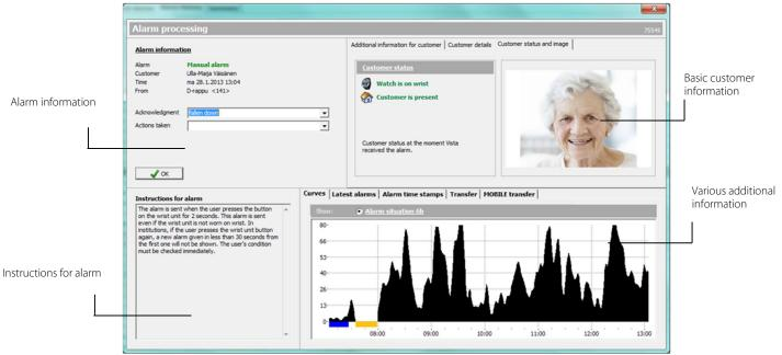
The alarm window can be closed by clicking on the OK button on the screen. The alarm is acknowledged by typing any text or selecting a predefined text into either one of the alarm's additional information fields, and then clicking on the OK button. Once you have entered the information, the fields are locked and you can no longer change the information.
